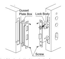
Install the door buckle plate on the door frame directly opposite the lock body. The hole of the buckle plate shall correspond to the tongue of to the lock body. If there is any deviation, it must be adjusted to the appropriate position.
