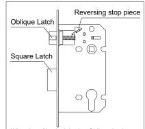
When installing lock body - Oblique latch should always be on top while square latch should at bottom. Oblique should face door closing way otherwise it has to be adjusted. Post this follow below steps:
